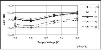
Figure 21. Gain vs. supply voltage, mode = high
